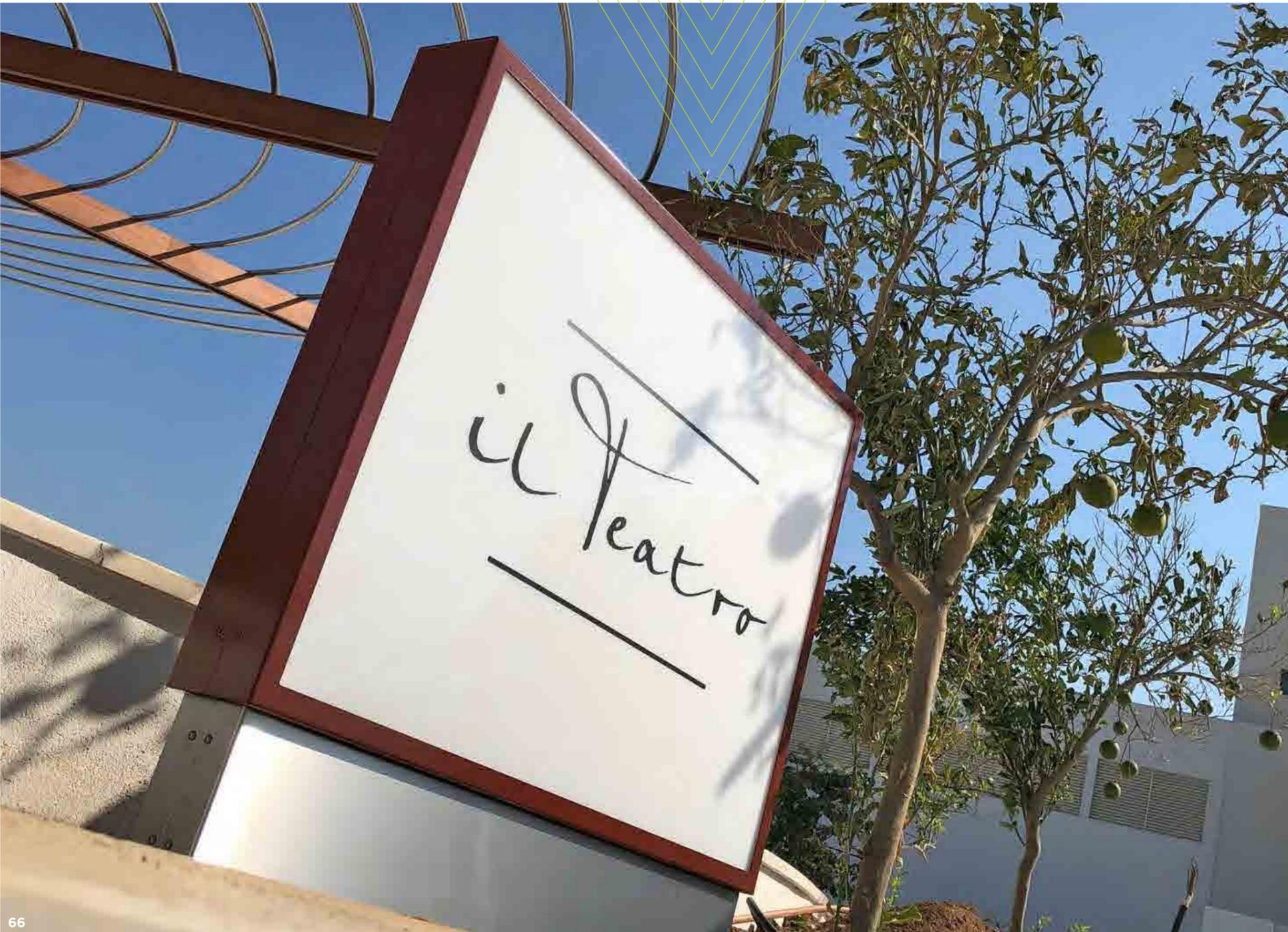
**THE TECHNICAL DETAIL:** The resort's external signage elements comprise branded entrance, directional and wayfinding signage and safety notices. Materials for the illuminated totem sign scheme include stainless steel subframes, stencil-cut aluminium trays that featured a specialist paint finish, push-through acrylic lettering and SloanLED illumination to set the scene for an unparalleled guest experience.
