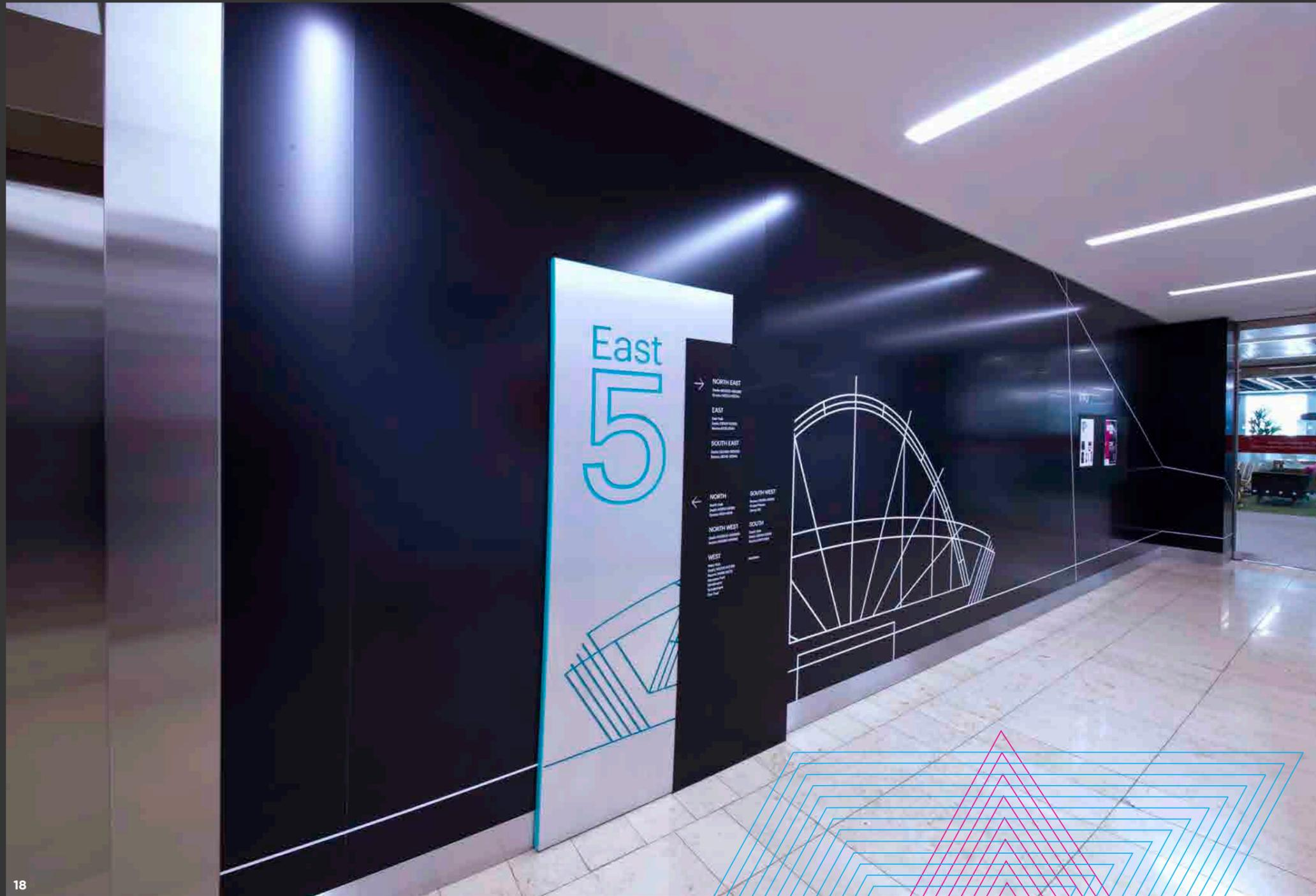
**THE TECHNICAL DETAIL:** Premium materials were utilised throughout this inventive project, including laser-cut acrylic with embedded LEDs, aperture-cut metal trays with push-through lettering, scratch-resistant, Lintec opti-clear manifestation film, Class O fire retardant Digimura supergraphics, birch-faced plywood icons, fluorescent vinyl details, internally illuminated LED light sheets, LG3880 high-tack vinyl and 30mm opal acrylic.
