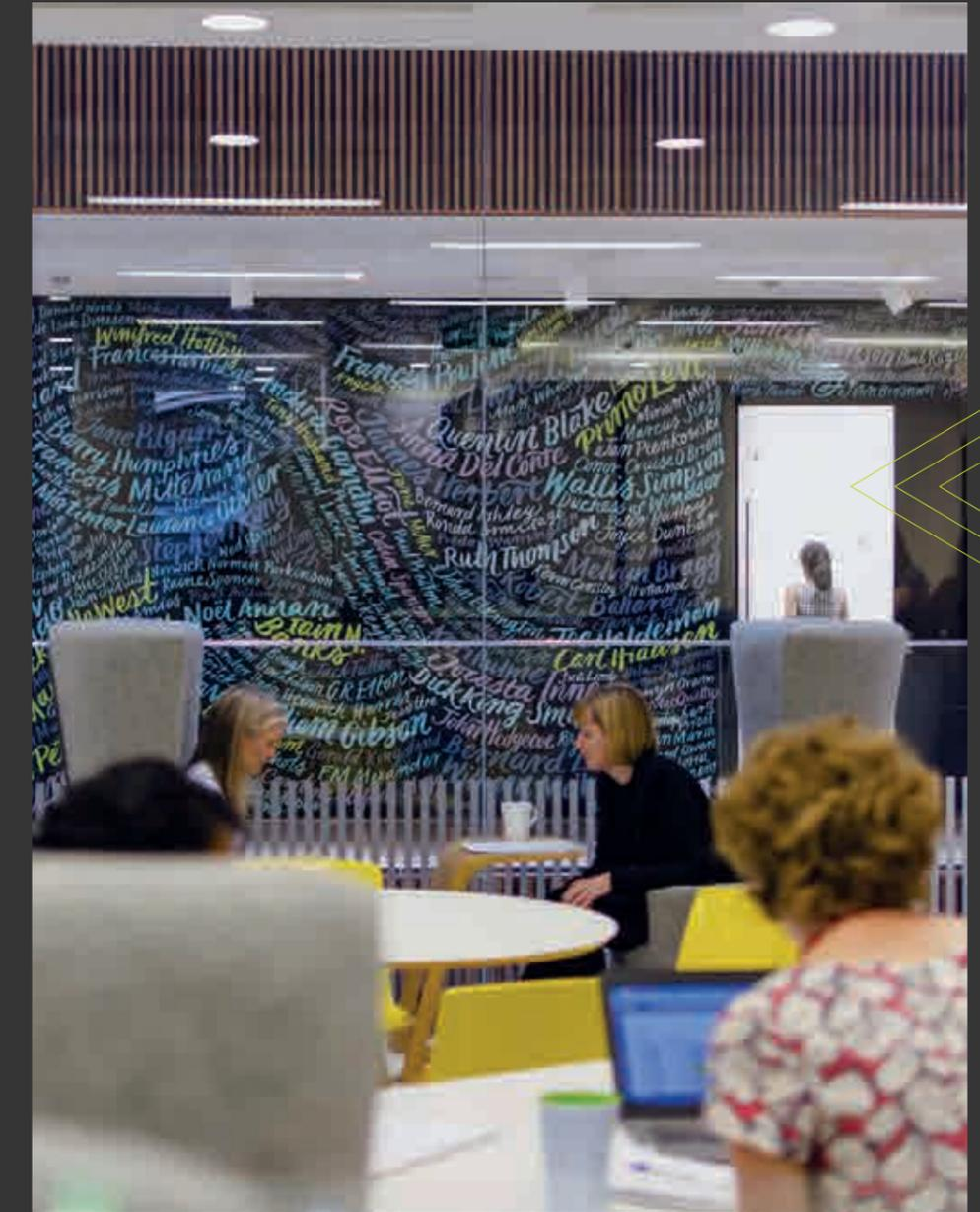
**THE TECHNICAL DETAIL:** This flagship Thames mural was digitally printed on Signbox's new HP Latex 360 printers on Class O, fire retardant LG 3880 high-tack vinyl. It took some 450 linear metres of the vinyl to cover every required wall surface and all had to be matt laminated, CAD-cut and weeded in readiness for application. Selecting the most suitable products that would adhere the material to acid-etched glass and preparing the surfaces were processes that were also critical to the finish.
